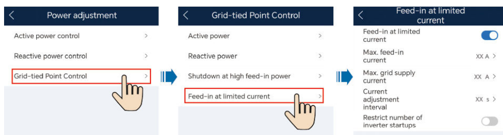
Figure 7-8 Feed-in at limited current
