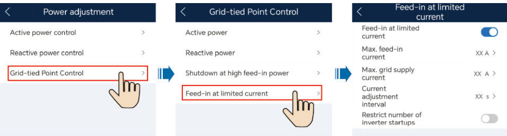
Figure 7-8 Feed-in at limited current
