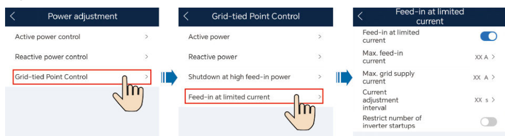
Figure 7-8 Feed-in at limited current
