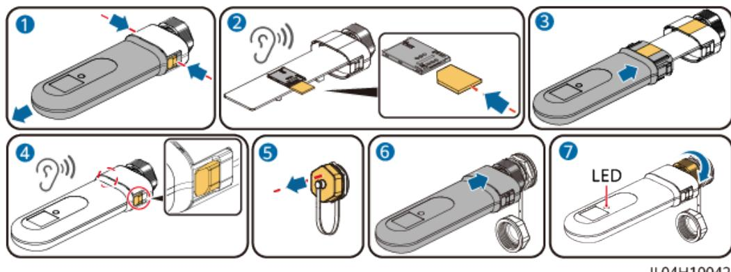
**Figura 5-44** Instalación de componentes antirrobo para el Smart Dongle
