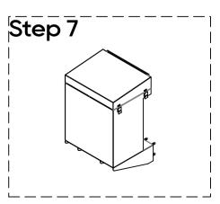
Place and lock the top cover to main cabinet by twisting the latches.
