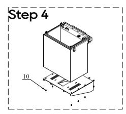
Install the main cabinet to wall by aligning Wall
