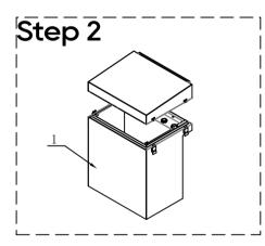
Untwist latches to remove the top cover of main cabinet.
