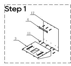
Fix the Wall Mounting Base and Wall Mounting Plate to wall with expansion screws by Positioning Board.
