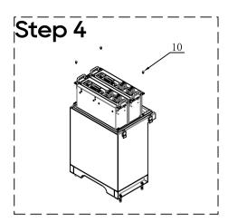
Place the batteris into cabinet as shown in picture and fix them to cabinet with M6 Screws.
