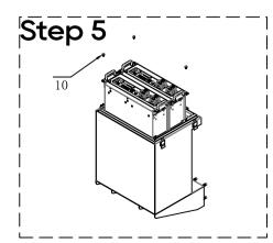
Place the batteris into cabinet as shown in picture and fix them to cabinet with M6 Screws.
