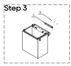
Fix the Wall Mounting Adapter to Cabinet with M4 Screws
