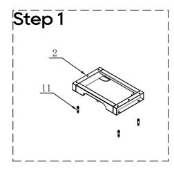
Fix the Floor Mounting Base with expansion screws
